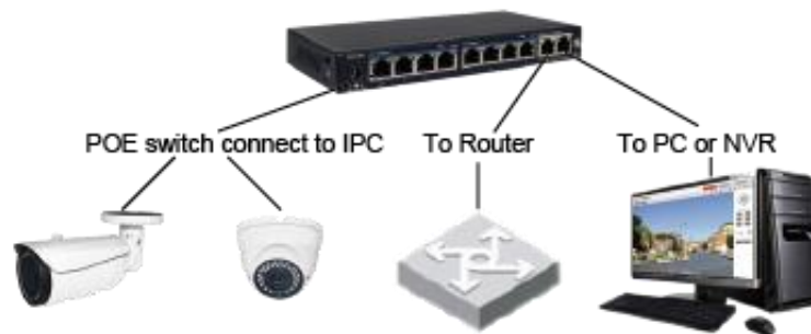
Pic 1-2 POE switch or router connection diagram
